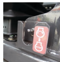
Emergency engine stop switch
