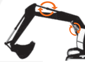
Boom & Arm Regeneration resulting in energy saving
