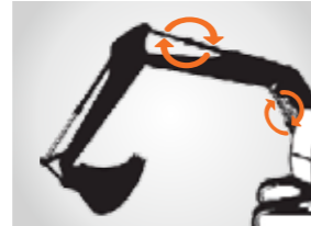
Boom & Arm Regeneration resulting in energy saving
