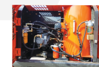
Ground level service access
